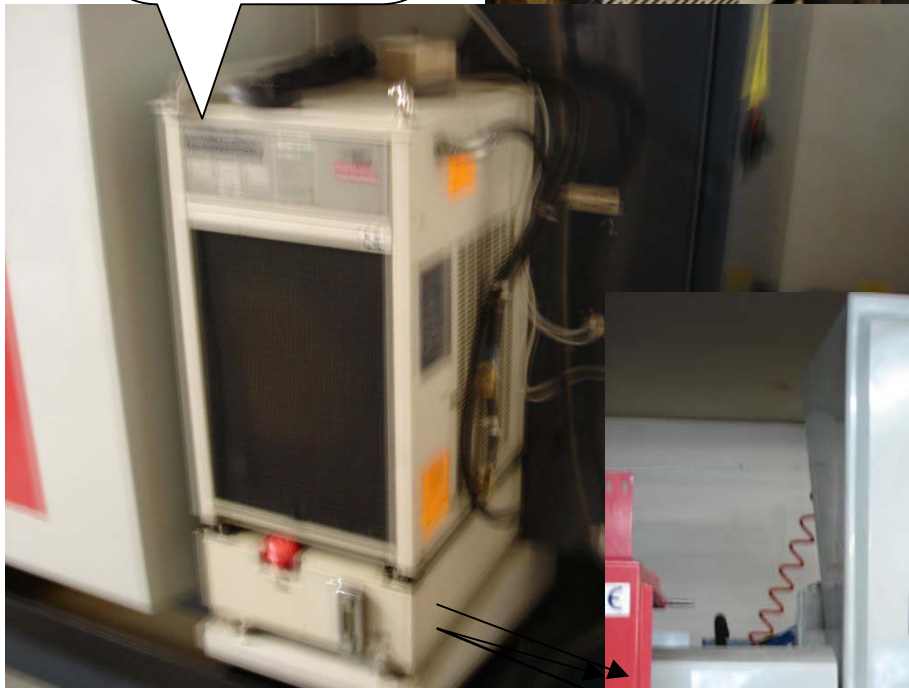
Spindle oil chiller system, 10.000 rpm continuos running !
